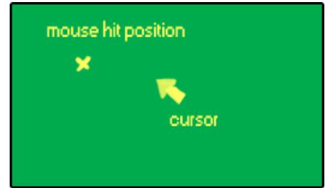
To solve this we have to know the difference between our screen resolution and scaleform movie resolution. Then multiply the percentual changes to our mouse position, making the mouse hit position update to our Scaleform cursor position.
